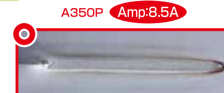
Stable weld bead obtained by fine amp control.
