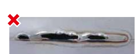
Burn-through caused by excessive heat input
